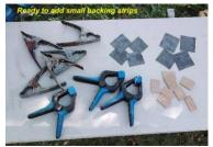
The last small side parts to add are 8 small squares that serve as backing strips at the edge of the original mast. These are simply cut from a pre-cured flat sheet of 200gsm bi-directional cloth. Their vertical dimension needs to close
