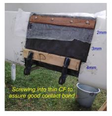
web at the lower edge. Note that this wing-piece must lay clear of the existing mast wall
