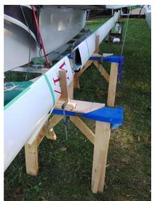
Start marking on the mast (see vertical green tapes in photo), a distance apart that will give you the original mast length. (It was 3ft in this case). Then place the two mast parts in the vertical supports, with the nose down, respecting the clearance you need to end up with the
