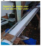
Once cured, paste over with fairing compound and do a final light fairing, making sure the fairing compound is thick enough that you do not remove any of the biaxial cloth. Then sand and paint 2 coats of polyester, and except for reassembly of the spreaders, the job is complete.
