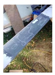
100mm greater than the new part, and slowly increasing the length of each added piece until the overlap over the existing mast is <u>at least</u> 100 times the thickness, ie: 400mm <u>minimum</u> for 4mm thickness. Before adding a 2<sup>nd</sup> layer, check carefully for any low spots, mark them with a chalk (see at left) and lay in some micro--balloon filler, as the target is to have the UNI laid as flat and straight as possible. Once dry, very lightly sand the
