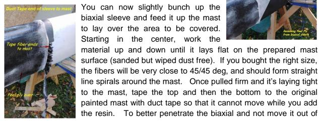
You can now slightly bunch up the biaxial sleeve and feed it up the mast to lay over the area to be covered. Starting in the center, work the
