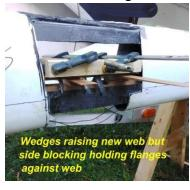
out at each end and also that the flanges are slightly longer. Both these attributes are important to blend in this relatively stiff I- beam to the side wall, without creating hard spots at the mast wall.
