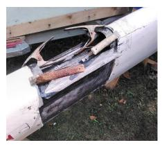
Once cleaned up, the mast is now rotated on the saw horses, bringing the nose uppermost so that the final backing strips can be added under the existing nose after first well-sanding the inside surfaces. See photo at left.
