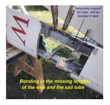
under the existing sail tube and fit up inside the existing wing sides with a good bonding surface.
