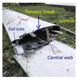
The mast snapped from 450lbs of boat falling on it from at *least* 8ft up (1/2 Beam plus beach clearance), a shock loading that is WAY higher than any possible sailing load.
