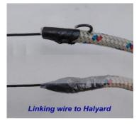
I now needed to remove the rope halyards so that they would not accidentally get 'bonded in'. So I attached the end of the halyards to a wire as shown above ..... by feeding a fence wire into the rope center, bending it back over before compressing it in place, and then added tape to create a cone shape that would feed readily through the mast wall guides.
