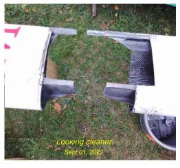
I now trimmed off the central web square across on both parts and also the sailtube, but did not cut them back more than is justified to find solid structure. You want the sail tube to be closest part when reassembling. I trimmed the sides along the
