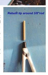
TIP to do this. Start by grinding a flat head on the stub and then drill out a 3/16" dia hole as
