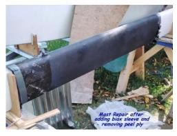
Remove the duct tape and sand down the upper and lower edges to blend the fiber ends into the original painted mast.
