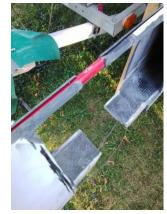
Arrange the other part of the mast at a height so that this *bolt* just slides cleanly into the upper part.
